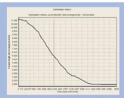
The X axis shows the wall cost, the Y axis the f açade length above target values [m]. The façade length considers individual floors. The red line indicates the chosen wall configuration for the graphics panel which can be saved for further noise map calculations.
