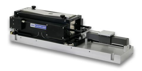
The **APS 500 ELECTRO-SEIS**® Air Bearing shaker is a long stroke, electrodynamic force generator specifically designed to be used for calibration and evaluation of accelerometers and other motion transducers. It provides excellent properties for low frequency excitation of such devices. The model consists of an air bearing driver attached to an air bearing load mounting table that allows payloads up to 3.0 kg (6.6 lb).
